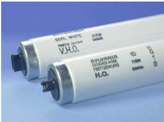
**Product** 25134**Number:****Order** F96T12/CW/HO/COLD TEMP**Abbreviation:****General** 110W, 96" MOL, T12 HO (800 mA) rapid start fluorescent**Description:** lamp, Cool White phosphor, 4200K color temperature, 60 CRI, labeled for cold temperature operation (below 60 degrees F) per EFACT. 12000 Avg rated life at 3 hrs/start**\* Full Case Required****Product Information**
