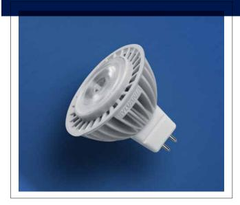
LED technology reduces energy and maintenance costs when compared to conventional light sources. They are free of UV and IR radiation minimizing discoloration and fading of materials. These lamps are dimmable down to 10%\* and are rated at up to 25,000 hours life with correlated color temperatures (CCT) of 2500K, 2700K and 3000K. They are available with a GU5.3 base and 25° and 36° beam angles.
